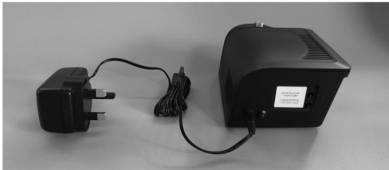
Plug the jack plug into the socket in the back, and the illuminator is now ready for connection.
